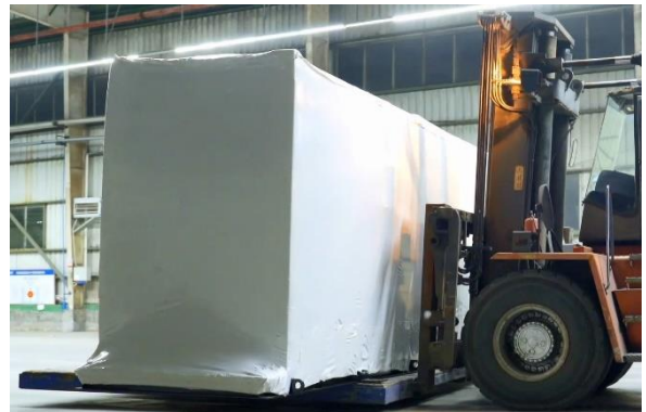
Figure 4-15 Skid-mount packing and transportation
